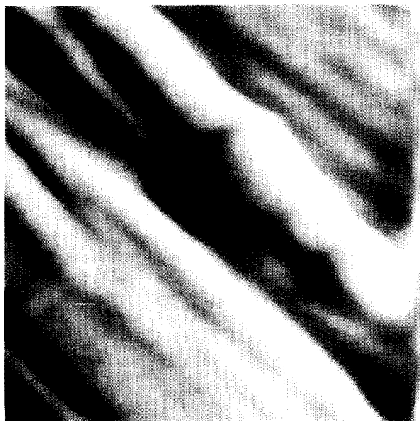
Figure 3 A low-magnification scan ( 1.1 \times 1.1 \mu\text{m}^2 ) of the x_2 plane, showing coarse fibrillar microstructure
